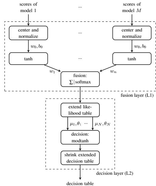
**Figure 2:** Structure of the Neural Network (NN)
