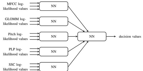
**Figure 5:** Structure of the Cascaded Neural Network
